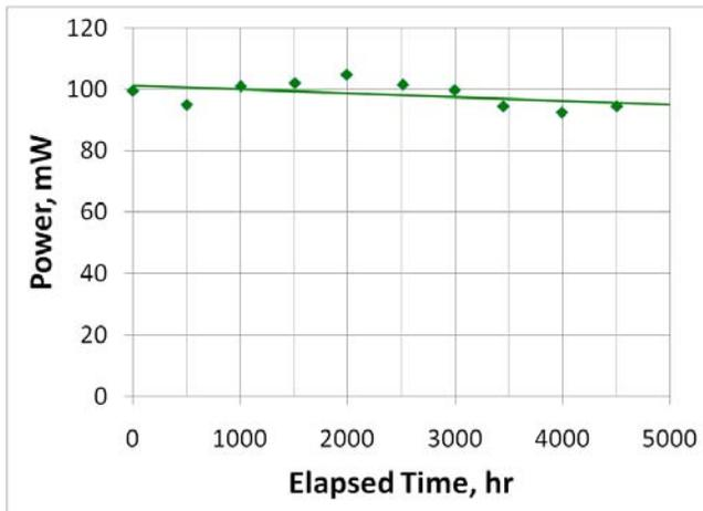
**Figure 2. Long-term output power test for a 100mW, cw Spectralus PPMgOLN microchip green laser source.**
