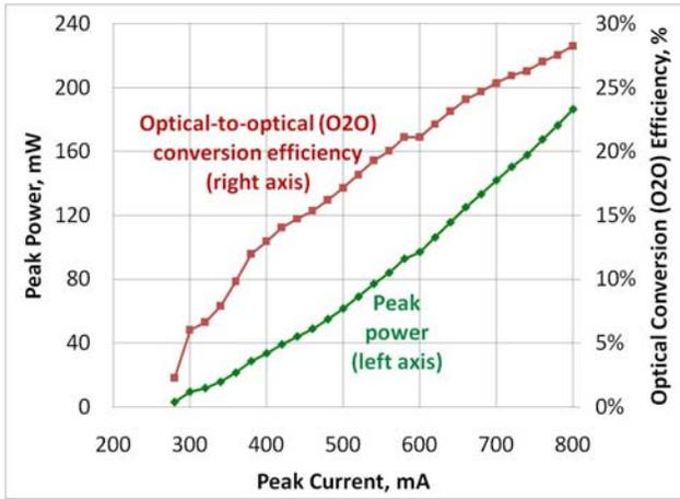
**Figure 4. Peak output power and optical-to-optical (808nm into 532nm wavelength) conversion efficiency as a function of current for a green laser source driven at 60Hz frequency with 33% duty cycle and set ambient temperature of 26°C.**
