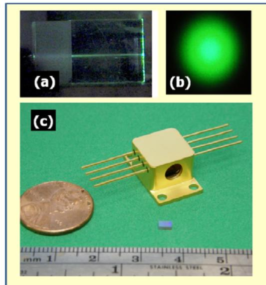
**Figure 1. (a) Top-view photograph of Spectralus' PPMgOLN-based microchip showing intracavity beam during laser operation; (b) green beam in the far field; (c) 8-pin mini-butterfly prototype package shown alongside with one US cent and a Spectralus microchip for scale comparison.**
