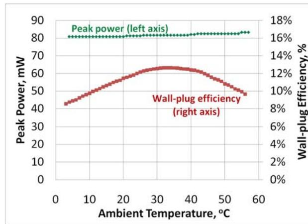
**Figure 3. Peak output power and wall-plug efficiency as a function of ambient temperature for a green laser source driven at 1.6kHz frequency with 25% duty cycle and set current of 380mA.**
